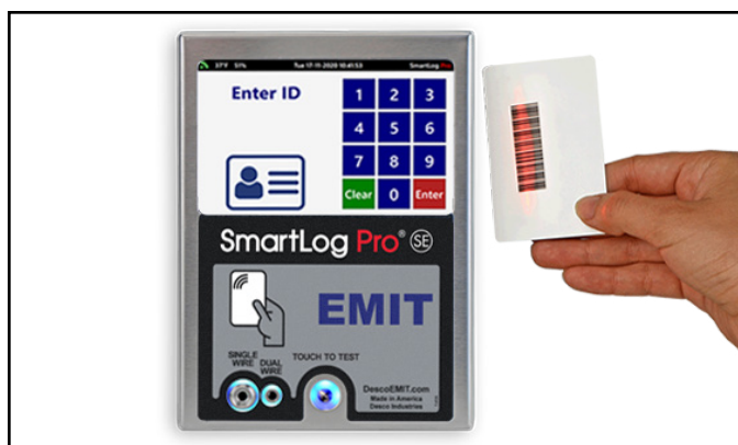
Figure 14. Using the barcode scanner
